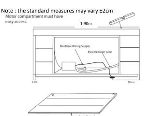
**IMPORTANT:** Important: The equipment must be connected to an exclusive and permanent power line capable to support installed power. Lighting and electrical receptacles must be located at least 1.5 meters from the equipment.
