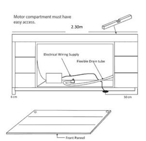
**IMPORTANT:** Important: The equipment must be connected to an exclusive and permanent power line capable to support installed power. Lighting and electrical receptacles must be located at least 1.5 meters from the equipment.
