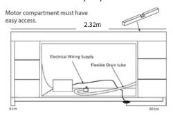
**IMPORTANT:** Important: The equipment must be connected to an exclusive and permanent power line capable to support installed power. Lighting and electrical receptacles must be located at least 1.5 meters from the equipment.
