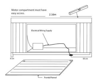
**IMPORTANT:** Important: The equipment must be connected to an exclusive and permanent power line capable to support installed power. Lighting and electrical receptacles must be located at least 1.5 meters from the equipment.
